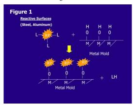
These substrates, which readily oxidize in air are said to possess reactive sites, typically characterized as having hydroxyl and oxide moieties protruding from the surface of the bulk metal. In other words, the cleaning process, which brought about the surface oxidation of the metal, has produced useful potential bonding sites for a reactive release system. The surface can be said to have been made "functional".
