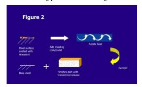
A conventional system would be spread over the entire surface of the mold by either wiping, brushing or spraying. Possessing no reactive sites, the system would wet and spread over the whole of the mold surface and remain essentially unchanged throughout the heat exposure cycle.
